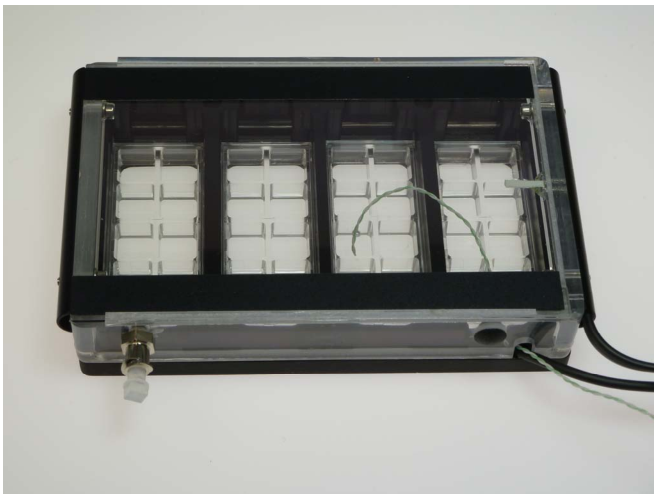
Figure 6: Sensor Placement for Temperature Calibration
