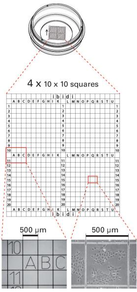
Microscopic images of the grid. Left: 4x objective lens brightfield without cells. Right: 10x objective lens phase contrast with rat fibroblast cells.
